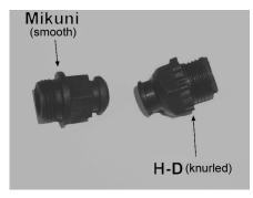
The Mikuni nut has a smaller hole where the cable fits and <u>must not</u> be used with the Harley choke cable.
