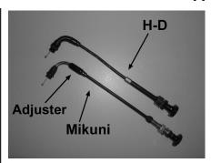
The Mikuni choke cable has an adjuster; the Harley cable does not. The Mikuni threaded section is steel while Harley's is plastic. The Mikuni cable has a hold-open detent; Harley's cable has a friction adjuster. The Mikuni knob has a small brass center while Harley's has the word "CHOKE" in white.
