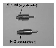
The Mikuni "Starter Plunger" and the Harley plunger are different and must not be interchanged. While they are very similar and both slide into the HSR carburetor, the <u>Harley plunger does not work in the HSR</u>. The Harley plunger does not seal and causes a severe rich condition.
