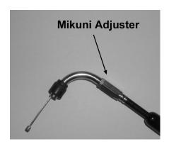
Mikuni's cable adjuster is covered by a rubber boot. There must be some free play in the cable. Any amount will do but there must be some to ensure that the choke plunger is fully bottomed.
