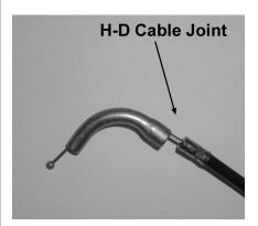
The Harley cable end may not completely bottom in the socket formed in the metal elbow. If the cable is not bottomed, the starter plunger does not seal. Poor mileage and a rich idle results.
