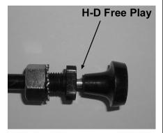
There must be some free play in the choke cable to ensure that the choke plunger is bottoming (sealing). Any amount of free play is okay, but there must be some.
